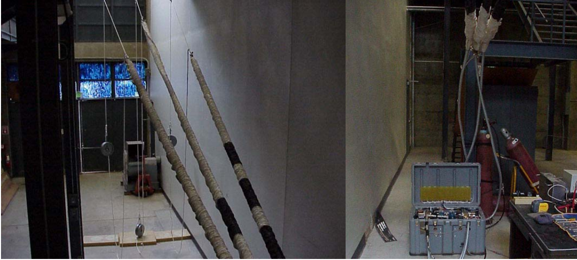
Figure 1.4 On the Left-PMAs 1 and 4 filled lifting 50 lb weights and PMA2 actuated. On the right- PMAs connected to the AGAS box.
