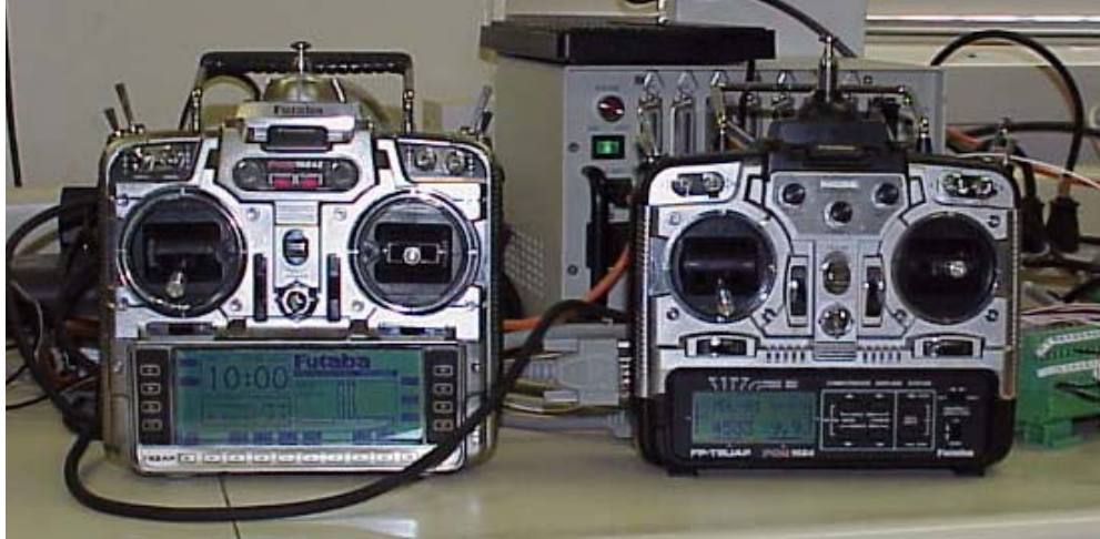
Figure A.8 Master (left) and Slave (right) w/ gray DB-9 cable in side of slave and black Trainer cable.
