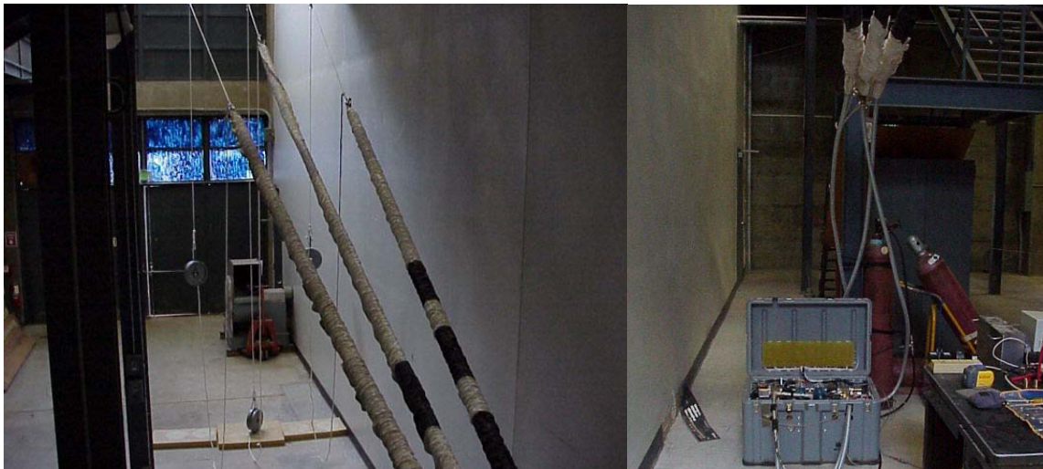
Figure A.34 On the Left-PMAs 1 and 4 filled lifting 50 lb weights and PMA2 actuated. PMA3 is missing and line is capped off; On the right- PMAs connected to the AGAS box.
