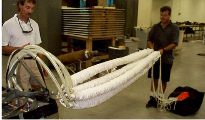
Figure 1.3 C-9 Parachute Pneumatic Muscles and system
