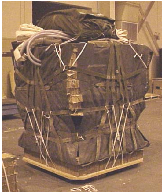
Figure 3.3 The AGAS package rigged for deployment
