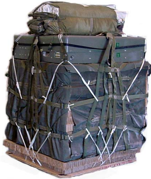
Figure 3.13 Serial/Autonomous AGAS package rigged for deployment
